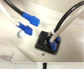
Unplug Black & White wires from Power Switch as shown to disconnect from Controller
