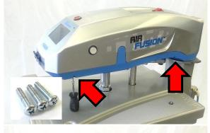
Remove three #8-32 x 3/4" Screws from Control Housing using Short #2 Phillips Screwdriver
