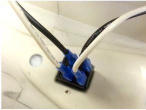
Plug in White & Black wires into Power Switch on opposite sides of the divider as shown to connect to Controller
