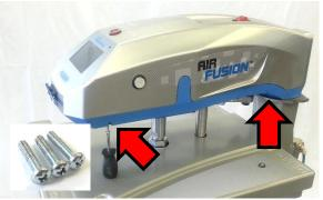
Replace Housing onto press and screw in three #8-32 x 3/4" Screws using Short #2 Phillips Screwdriver
