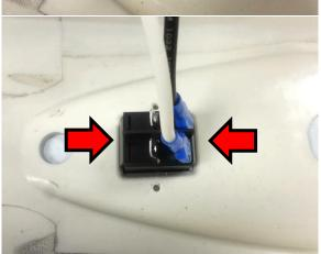
Squeeze retaining clips together to release switch from housing
