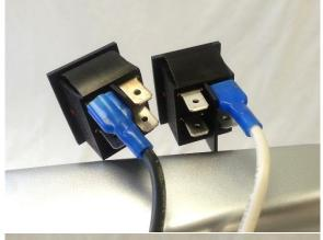
Transfer wires from old Power Switch to new, one at a time to ensure each wire attaches to the correct terminal
